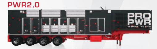
THE PWR2.0 IS THE OPTIMAL SOLUTION FOR GENERATION CAPACITY, OFFERING BOTH ECONOMIC EFFICIENCY AND ENVIRONMENTAL SUSTAINABILITY. IT IS METICULOUSLY DESIGNED TO MEET THE CRITICAL REQUIREMENTS OF PROJECTS DEMANDING HIGH RELIABILITY AND AVAILABILITY. THE PWR2.0 IS POWERED BY THE WAUKESHA 9394S5 RICH BURN GENERATOR SET, A PROVEN INDUSTRY STANDARD.
